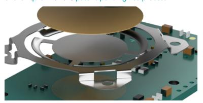
The filling level is determined by the hydrostatic pressure, which is measured with an inductive pressure sensor. The pressure sensing element is a special flat spring interacting with a spiral coil on the PCB.
