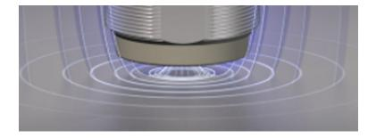
This change in impedance produces an electrical signal that is proportional to the distance between the target and the sensor coils. The use of 2 coils results in a fully differential system that is very robust against external interference.
