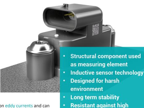
The measuring principle is based on eddy currents and can detect changes in geometry in the nanometer range. High-frequency alternating current flows through 2 coils built into a sensor housing. The electromagnetic coil field induces eddy currents in the conductive target, which changes the resulting alternating current resistance of the coils.
